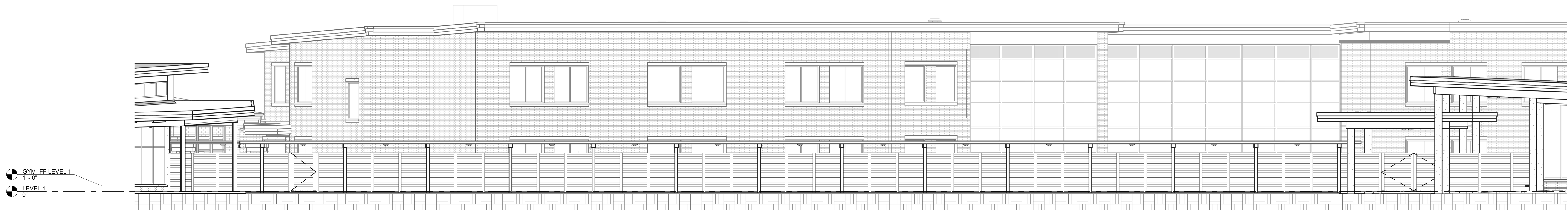
4 GYMNASIUM TO ADMINISTRATION WALKWAY ELEVATION - NORTH SCALE: 1/8" = 1'-0"
